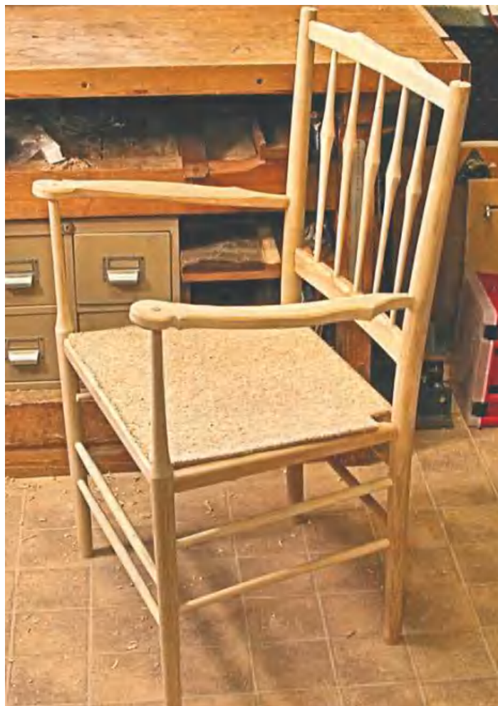
◀ Pic. 1 The unfinished chair showing the modified top rail
